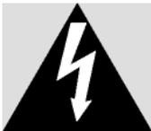
The arrow-end lightning symbol inside the equilateral triangle informs that in the context of the product, there is enough amount of 'not insulated' dangerous voltage to cause an electric shock.
