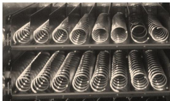
The vending machine has 6 Trays (+1 optional). In the machines with an optional cooling unit, cold products can be placed in the bottom three trays. To avoid any damage, place any breakable and heavy products into the trays close to the dispense compartment.
