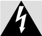
The arrow-end lightning symbol inside the equilateral triangle informs that there is high amount of 'un-insulated' dangerous voltage to cause an electric shock inside the product.
